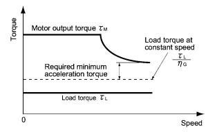
Figure 7.4 Example Study of Required Minimum Acceleration Torque
