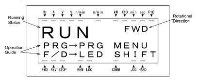
Figure 3.3 Display of Running Status
