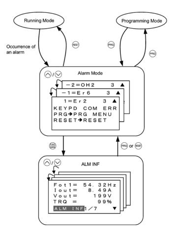
Figure 3.33 Menu Transition in/from Alarm Mode
