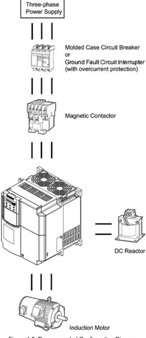
Figure 1.5 Recommended Configuration Diagram
