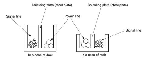
Figure A.7 Separate Wiring
