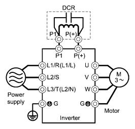
Figure 6.7 Applying a DC Reactor (DCR)
