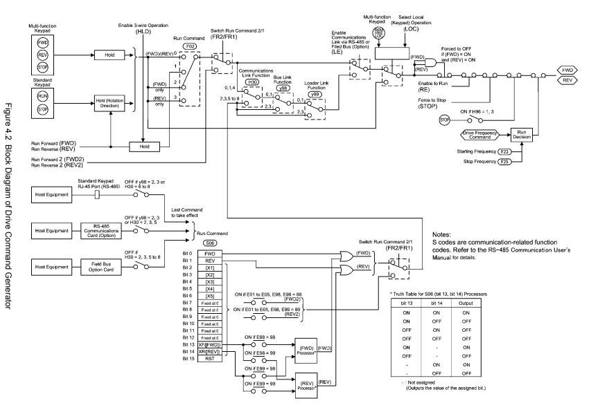
Figure 4.2 shows the processes that generate the final drive commands (FWD: Drive the motor in the forward direction and REV: Drive the motor in reverse direction) through the various run commands and switching steps by means of function codes.
