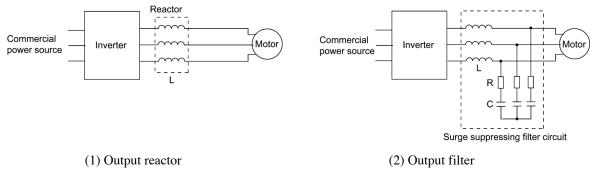
Figure C.3 Method to Suppress Surge Voltage
