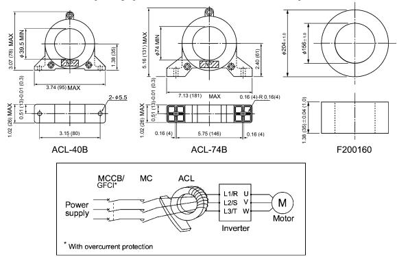
Figure 6.10 Dimensions of ACL and Application Example
