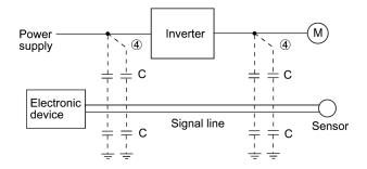
Figure A.5 Electrostatic Induction Noise
