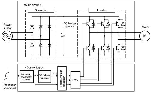
Figure 1.4 Schematic Block Diagram of FRENIC-Eco
