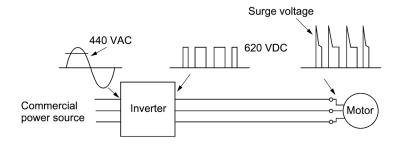
Figure C.1 Voltage Wave Shapes of Individual Portions
