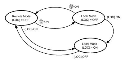
Figure 3.5 Transition between Remote and Local Modes
