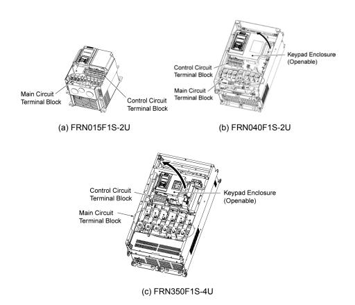
Figure 2.2 Terminal Blocks and Keypad Enclosure Location
