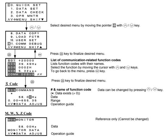
Figure 3.29 Menu Transition for Communication Debugging
