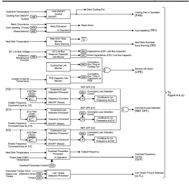
Figure 4.4 (b) Block Diagram of Digital Output Components (Internal block)
