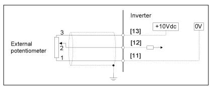
Figure 6.11 External Potentiometer Dimensions and Application Example
