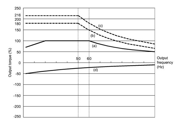
Figure 7.2 Output Torque Characteristics (Base frequency: 60 Hz)
