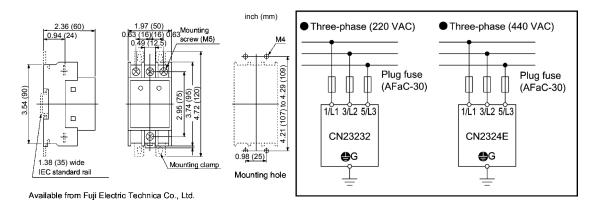
Figure 6.4 Arrester Dimensions and Application Examples
