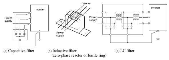
Figure A.10 Various Filters and their Connection
