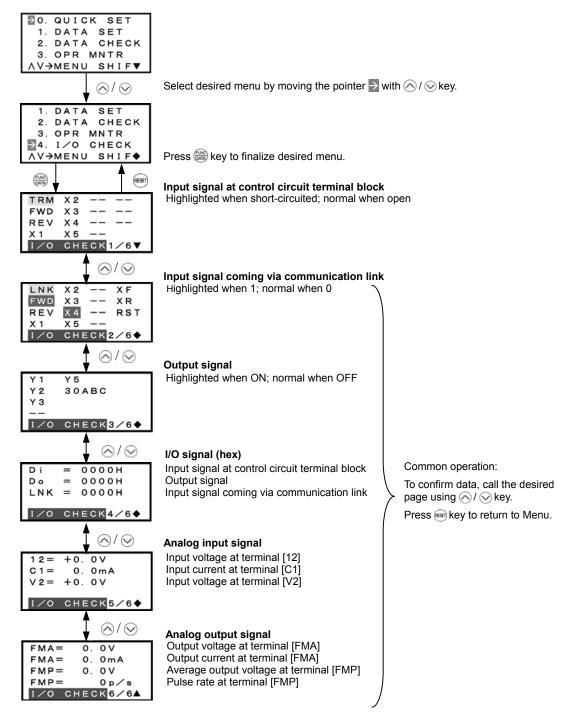
Figure 3.15 Menu Transition for "I/O CHECK"
